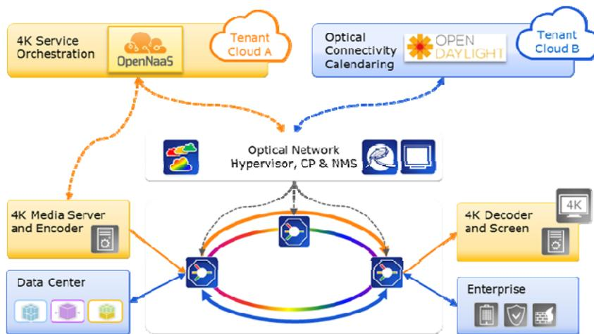
representations of the underlying transport network and exports that abstracted network to client SDN controllers. An abstracted network can be exposed as a single node or multiple nodes with abstract links. From the perspective of the exposed SDN interface the Network Hypervisor acts as one or more (virtual) nodes.
